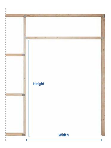
The Rocket Pocket kit will adapt to almost any stud dimension HOWEVER, the stud immediately above the frame must be 2x4. You can add layers of plasterboard to this to then obtain the wall thickness you require. Bare in mind the jamb dimensions will change accordingly (page 23).
